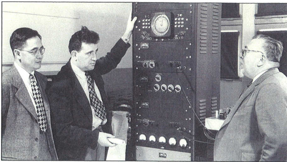
In 1948, former RadLab staff member Professor Jerome B. Wiesner (center) discusses results from the first electronic analog correlator with Professors Yuk Wing Lee (left) and Norbert Wiener. Professors Wiesner and Lee were instrumental in translating Professor Wiener's theory of nonlinear systems into practical applications. By combining the methods and techniques of mathematicians and communication engineers, the study of communication theory in RLE was not confined to electrical systems. (RLE file photo)
