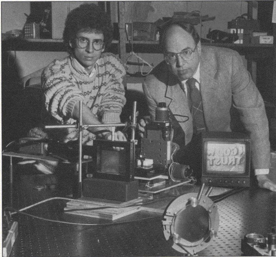
Professor David H. Staelin (right) and graduate student Howard R. Stuart adjust a positioning and imaging device designed to explore the limits to precision and speed when measuring or "reading" the detailed shapes of small mechanical objects. Because desired accuracies are on the order of microns, problems arise in the micro-optical behavior of surfaces, precision micro-distance measuring algorithms, and computational efficiency. Similar apparatus is being developed to address the issues of duplicating or "writing" the objects which have been "read." The monitor in the photograph displays the reversed image of a quarter's imprint "In God We Trust." (Photo by John F. Cook)
