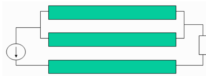
Figure 3.10: Simple example to describe high frequency effects such as skin and proximity effects. Conductors are 6 mm long, 1mm wide and 1mm far apart from each other. The two conductors on top are two possible return paths for the current on the conductor on the bottom.
