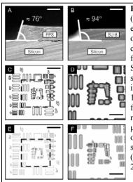
Figure 1: Resolution tests. (A) & (B) show scanning electron micrographs (SEMs) of sidewall angles in a direct comparison between patterns formed using PPS and SU-8. Scale bar 25 um. (C) and (E) show bright-field microscopy images of the standard USAF 1951 resolution test pattern for the case of PPS and SU-8 respectively. Scale bar 50 examines the (D) outlined region in (C) and (F) surveys the outlined region in (E) in closer detail. Scale bar 25 μm.
