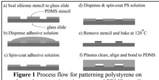
glass substrates using micropatterned PDMS stencils.
