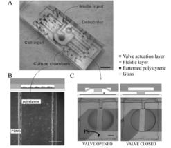
Figure 2 Applications of micro-patterned polystrene. (A) Image of a two-layer microfluidic device that incorporates cell culture chambers and normally closed valves. Scale bar 5 mm. (B) Top view of a MPPS culture chamber with NIH-3T3 mouse fibroblasts. Scale bar 150 um. (C) Schematic of valve cross section (C, top). PS patterned valve seat prevents PDMS valve membrane from bonding (C, bottom). Scale bar 200µm.
